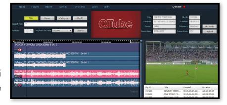
Leveraging the Quantel® server technology, Fairlight's Gateway accesses Quantel® compositions directly, with no rendering or video file import required. Frame accurate playback, jogging and scrubbing is instantly available over a local LAN network or even over the internet.
